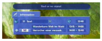
"Weak signal or no signal" indicates that an error has occurred in the reception system or in the receiver settings, or that the transponder is not sending. The channel identifier shows a satellite antenna instead of the  $\vec{\iota}$ . Check the Sat IF connection and the LNB configuration. The list of service settings at the end of this manual can be used to help you do this.
